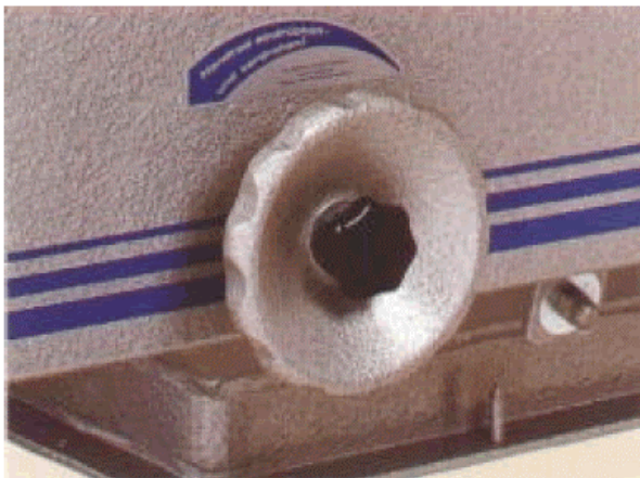
Handwheel quick adjustment for Minor S, Norma S, Plus and all Universal models from 2,2 kW upwards
